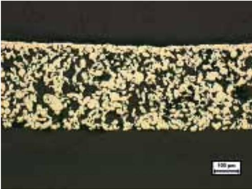
Light optical microscopy picture of a cross section of a sintered metal powder sheet with a gradient porosity structure.
