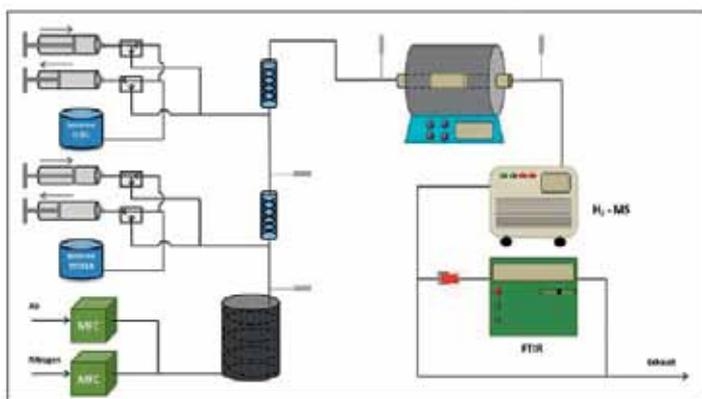
Miniature catalyst activity evaluation test rig. MFC: Mass Flow Controller; MS: Mass Spectrometer; FTIR: Fourier Transform Infra-Red Spectrometer.
