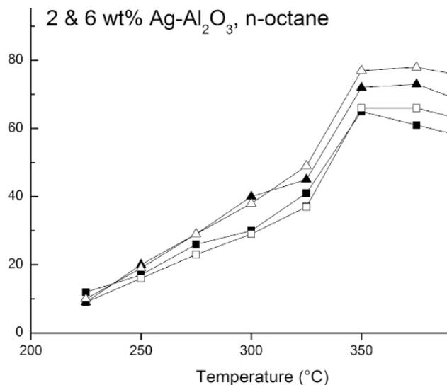
NO<sub>x</sub> conversion as a function of temperature over various silver-alumina catalysts, using bio-diesel (NExBTL) as reducing agent.
