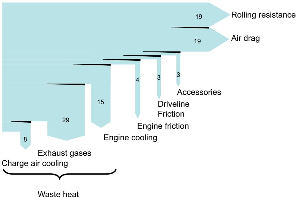
Schematic illustration of energy distribution for a long-haul truck running at 90 km/h on flat road.
