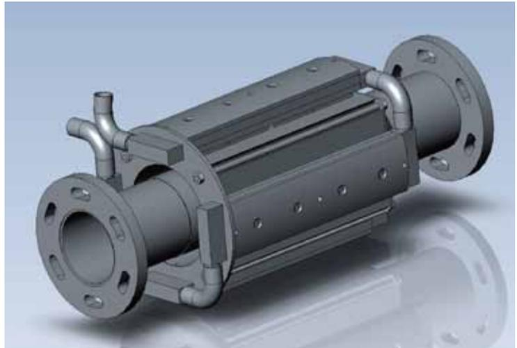
Thermoelectric generator designed for use in the integrated system.
