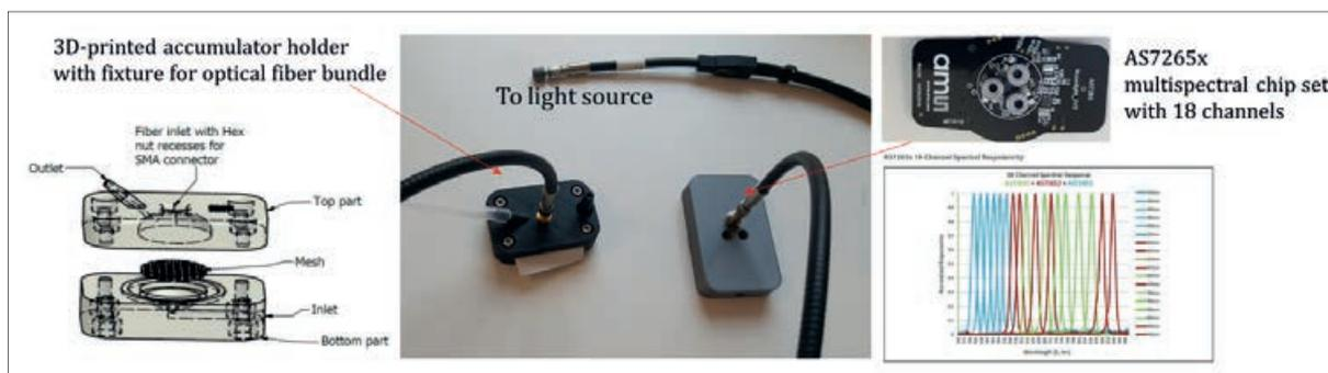
**FIGURE 5.** An optical fibre filter cartridge for monitoring of accumulation during filter operation.
