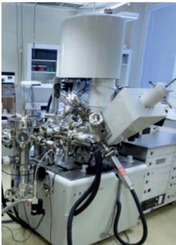
**FIGURE 4.** The XPS instrument at RISE was used to analyze the surface chemical composition of Mistra TerraClean materials.
